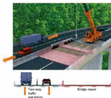
Replacement image of a floor panel
